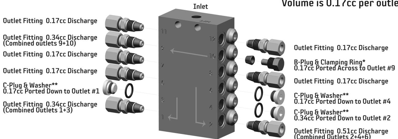
\*\*Note: C-Plugs port volume down to the adjacent outlet away from the inlet (C-Plugs cannot be used in outlets 1 or 2)
