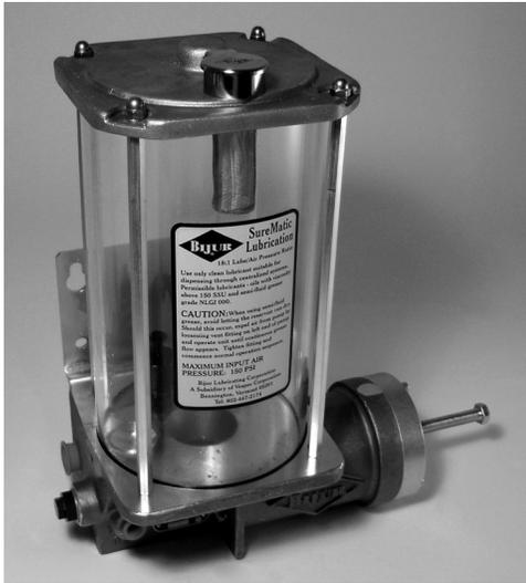
The SureMatic Lubricator comprises a piston discharge pump actuated by air, controlled by an electric solenoid 3-way valve. Models are available to handle grease and oil. Low level switch is standard on all models.
