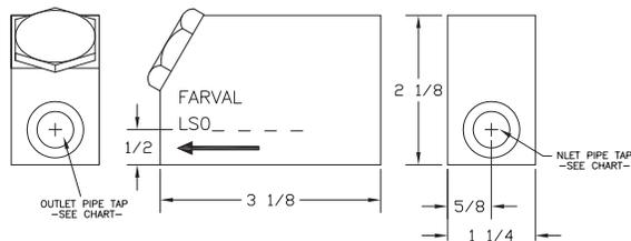
1. LS Line Strainers remove foreign particles from grease and oil lines in lubricating systems. Withstand up to 5000 psi working pressure non-shock.
