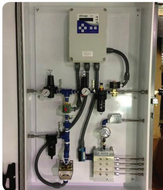
*Automatic Grease System in Enclosure*
